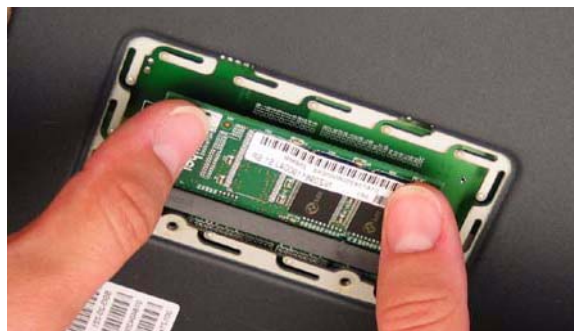
Figure 21: Inserting the Memory Module
